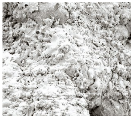
SEM pictures of a HA-sprayed surface
